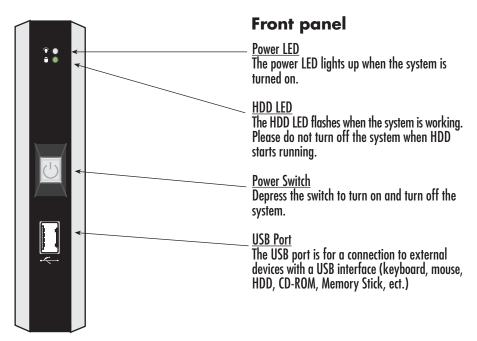
Figure 3. Ultra-Thin System - Front panel
